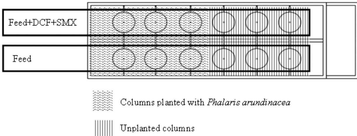
Figure 1. The scheme of the lab scale system used in the experiment
