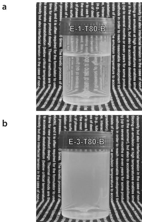
Figure 5. Macroscopic picture of emulsions E-1-T80-B (a) and E-3-T80-B (b).
